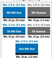
MIG aluminum welding uses optional Spoolmate 100 and 4000 series aluminum wire OR Spoolmate 150 and either 4000 or 5000 series aluminum wire.
