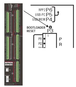
**Figure B-1.**Bootloader Reset on CPU panel
