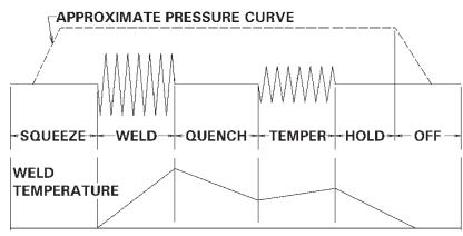
Figure 9-9. Quench-Temper with Chained CYCLE MODE
