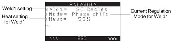
**Figure 5-26.** *WELD1 in Phase Shift mode*
