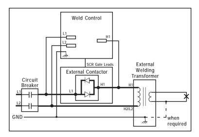
Figure 4-8. Schematic for External SCR
