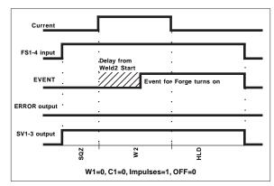
**Figure 9-16.** Forge Delay Weld using Events
