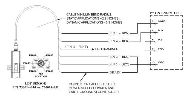
Figure 4-11. Linear Displacement Transducer Sensor wiring diagram
