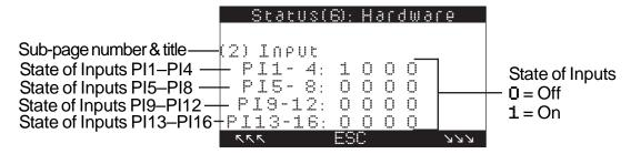
Figure 5-13. Hardware Inputs
