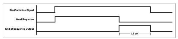
**Figure 9-3.** End of Sequence in Spot operation
