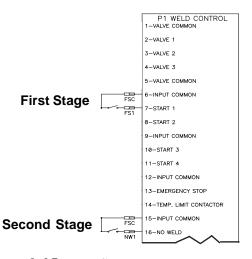
**Figure 9-25.** Two Stage initiation in Brazing mode
