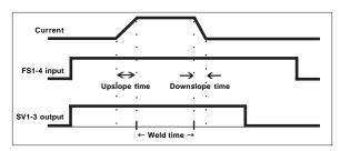
Figure 9-10. SLOPE function in Spot Weld
