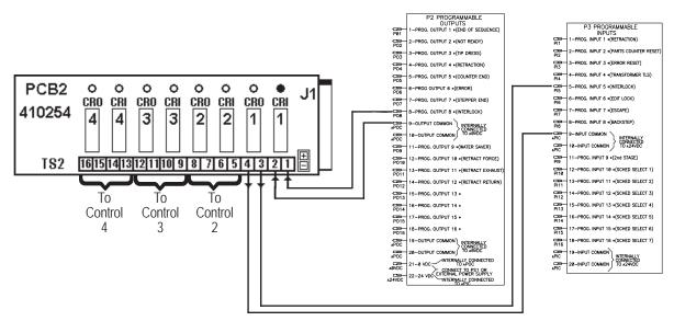
Figure 9-56. Welder Interlock connections
