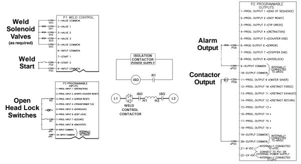
Figure 9-35. Head Lock wiring
