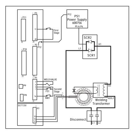
Figure 6-1. Basic connections
