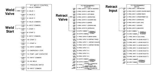
**Figure 9-30.** Maintained Retraction connections
