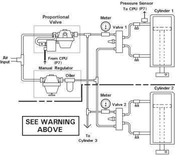
**Figure 9-61.** IPSC System with Proportional Valve and Sensor in Single function or Cascade control
