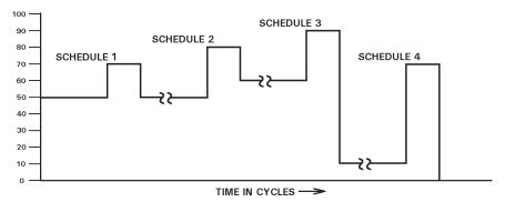
Figure 9-24. Seam mode with timed heats
