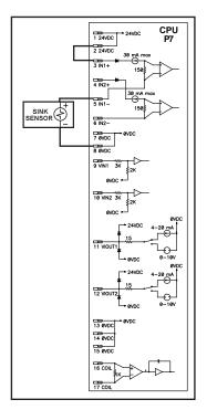
**Figure 9-69.**Sinking Sensor Wiring Logic
