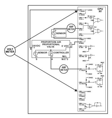
Figure 9-71. IPSC block diagram
