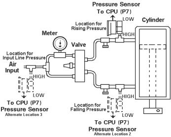
The Differential Pressure Sensor has two connections, one high and one low. This sensor can be used as a single ended sensor by using only the high pressure port (Figure 9-64).
