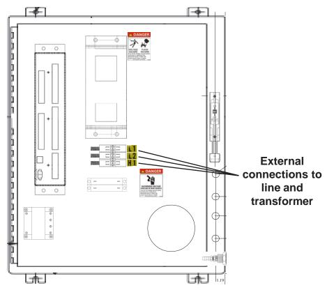
Figure 4-7. Wiring Diagram for External SCR Contactor
