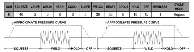
**Figure 9-6.** Spot with Repeat CYCLE MODE
