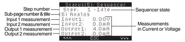
Figure 5-10. Sequencer Analog Inputs and Outputs
