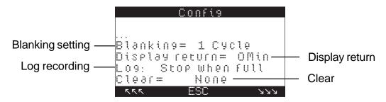
**Figure 5-50.** *Configure Menu – Sample Display 7*
