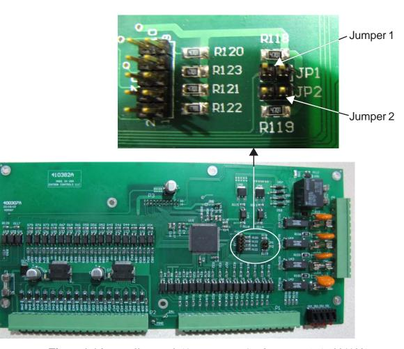
**Figure 1-16.** *Installation of I/O Expansion Card Jumpers (P/N 331139)*
