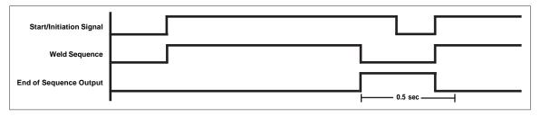
**Figure 9-4.** *End of Sequence with new start/initiation signal*
