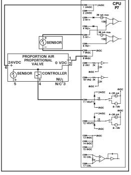
**Figure 9-66.** *IPSC Wiring Logic – Proportion-Air*
