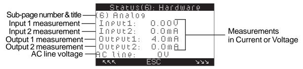
**Figure 5-14.** *Analog Inputs and Outputs*
