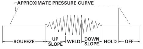
Figure 9-13. SLOPE with Chained CYCLE MODE
