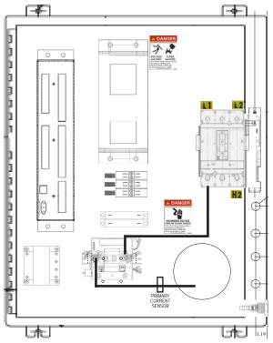
**Figure 2-1.** Installation of Style "N" Cabinet – 150/300 Amp Contactor
