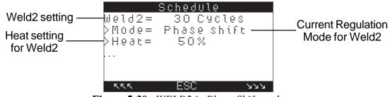
Figure 5-30. WELD2 in Phase Shift mode
