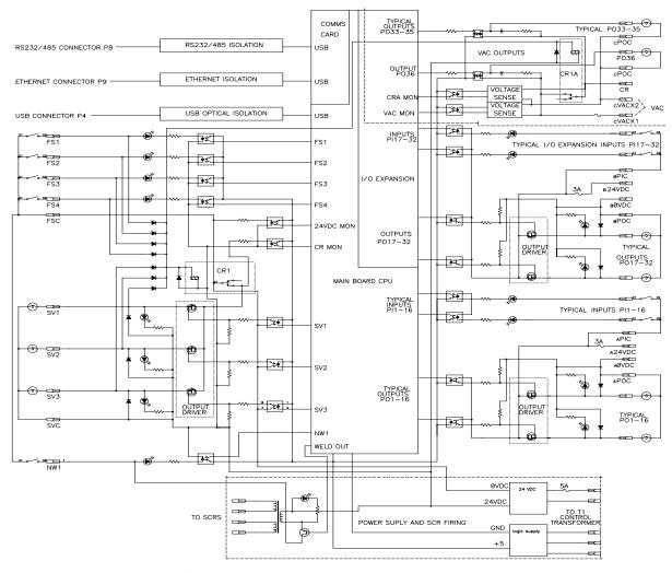
Figure 3-1. Typical input and output schematic
