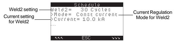
Figure 5-31. WELD2 in Constant Current mode
