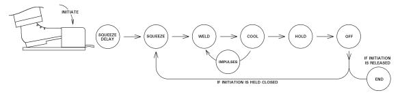
Figure 9-26. SQUEEZE DELAY operation
