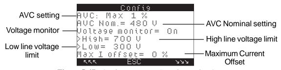
**Figure 5-47.** *Configure Menu – Sample Display 4*
