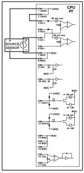
**Figure 9-68.**Sourcing Sensor Wiring Logic
