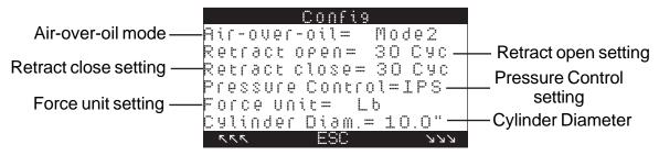
**Figure 5-45.** Configure Menu – Sample Display 2
