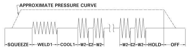
Figure 9-22. Intermittent Seam mode using WELD1/COOL1
