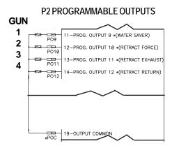
Figure 9-37. Multiple valve connection
