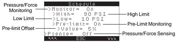
Figure 5-23. PRESSURE/FORCE MONITORING
