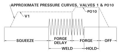
Figure 9-17. Forge Delay using Events
