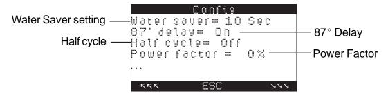
**Figure 5-48.** Configure Menu – Sample Display 5
