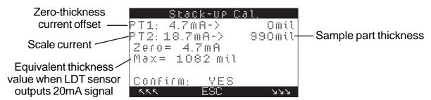
Figure 5-55. Stack-up Calibration sub-menu
