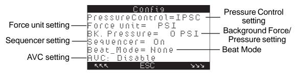
**Figure 5-46.** Configure Menu – Sample Display 3
