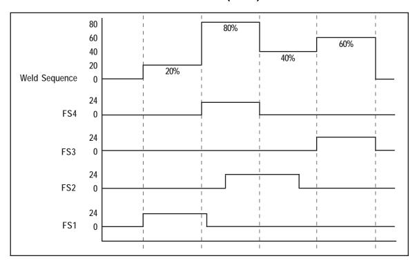
**Figure 9-23.** *Seam mode with multiple initiations*
