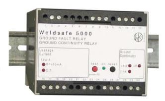
The Weldsafe 5000 combination ground fault current and ground check relay has been designed to provide sensitive ground fault protection and continuous ground checking for ac, 50-60 Hz manual transguns in accordance with RWMA Bulletin 5 standards.
