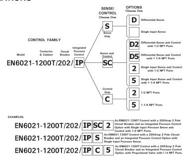
**Figure 9-58.** *IPSC configurations*
