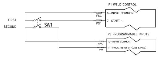
**Figure 4-9.** Single two-stage foot switches connection diagram
