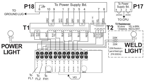
**Figure 4-3.** Power Supply schematic
