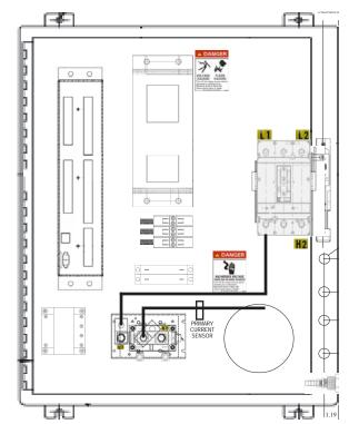
**Figure 2-2.** Installation of Style "N" Cabinet
