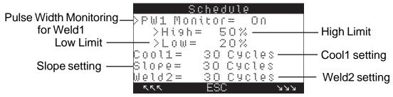
Figure 5-29. PULSE WIDTH MONITORING for WELD1
