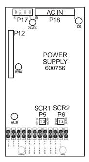
**Figure 4-2.** Power Supply connectors
