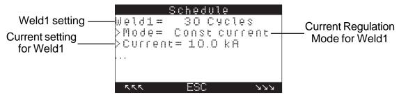
Figure 5-27. WELD1 in Constant Current mode
