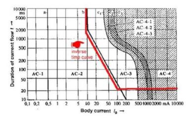
Weldsafe 5000 Ground Fault Setting 2 reaction time
