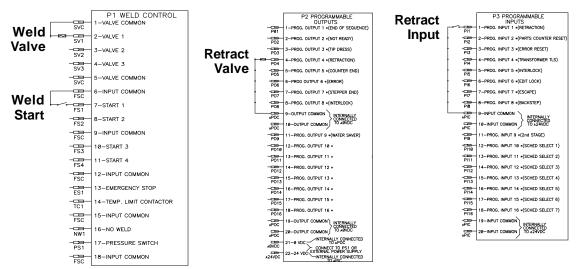
Figure 9-28. Momentary Retraction connections
