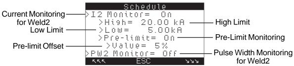
Figure 5-32. CURRENT MONITORING for WELD2
