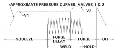
**Figure 9-15.** Forge Delay with Chained CYCLE MODE
