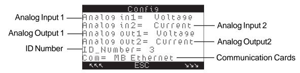
**Figure 5-49.** Configure Menu – Sample Display 6
