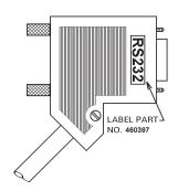
**Figure A-2.** *RS232 Connector labeling*
