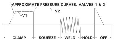
Figure 9-14. Butt Weld with Chained CYCLE MODE
