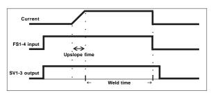
Figure 9-18. Continuous Seam Weld
