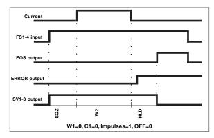
Figure 9-1. Basic Spot Weld—No Weld Faults
