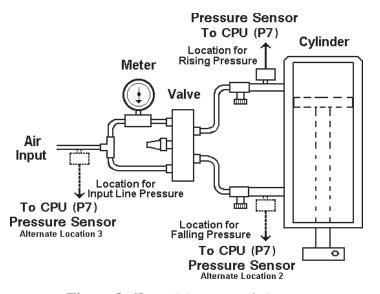
**Figure 9-62.** *IPS System with Sensor*
