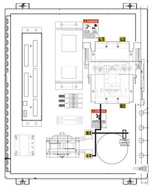
**Figure 2-3.** Installation of Style "N" Cabinet – 1800/2200/3200 Amp Contactor
