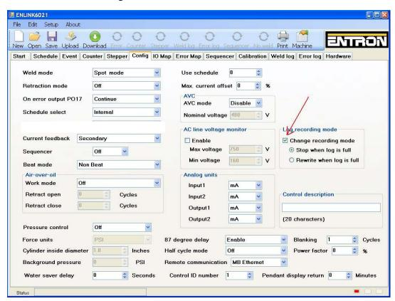
Figure 5-52. LOG RECORDING MODE using ENLINK
