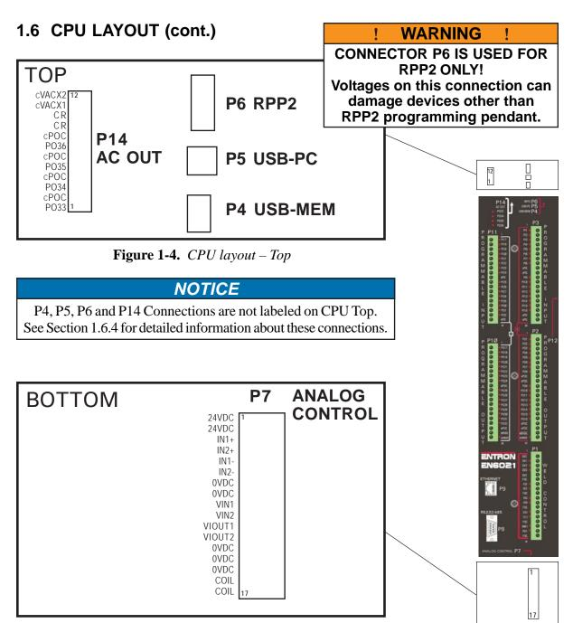
**Figure 1-5.** *CPU layout – Bottom*
