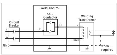
**Figure 4-6.** Power connections
