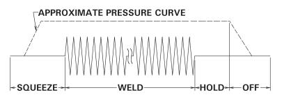
Figure 9-19. Continuous Seam mode
