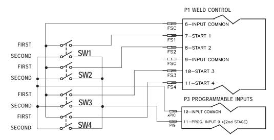
**Figure 4-10.** *Multiple two-stage foot switches connection diagram*
