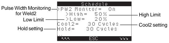
**Figure 5-33.** *PULSE WIDTH MONITORING for WELD2*
