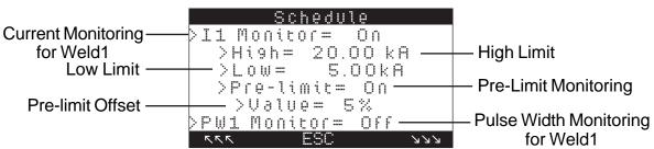
Figure 5-28. CURRENT MONITORING for WELD1
