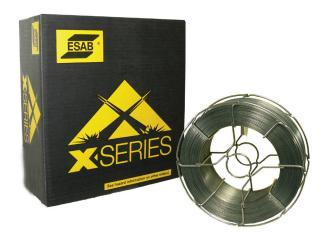
Dual Shield 710X is an all-position flux cored wire for general purpose welding. It provides outstanding operator appeal with an easily controlled arc, improved operation at both lower and higher current levels, minimal spatter and easily removed slag. Dual Shield 710X is designed primarily to be used with 100% CO2 gas mix, especially for applications where weld joint restraint is high. Applications include railcars, barges, civil construction, light equipment and general fabrication.
