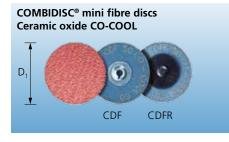
COMBIDISC<sup>®</sup> mini fibre disc with ceramic oxide grain is designed for very hard-to-machine materials such as stainless steel, Hastelloy<sup>®</sup>, Inconel<sup>®</sup>, titanium etc. Active additive fillers in the coating increase the stock removal rate substantially while preventing loading and heat build-up.
